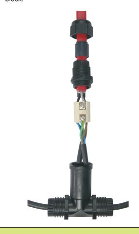
Slide the ceramic terminal block into the body, pushing it and simultaneously pulling on the round cables. Then screw the body of the cable gland A without having entered the flat cable silicone gasket.
